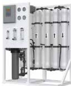
**L4 RO SYSTEM** | Produces high purity water by reducing contaminants such as dissolved minerals, particulates, and organic impurities using a reverse osmosis membrane system. Complete, skid mounted, pre-plumbed, pre-wired reverse osmosis (RO) system for quick installation and start-up.
